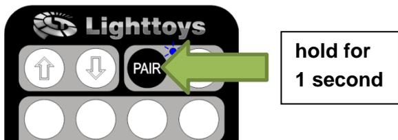
First, press and hold the PAIR button for 1 second. The indicator LED will start blinking. This shows the remote has entered pairing mode.
