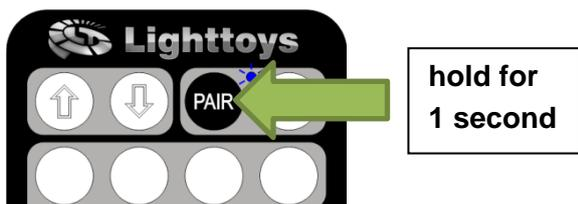
First, press and hold the PAIR button for 1 second. The indicator LED will start blinking. This shows the remote has entered a pairing mode.
