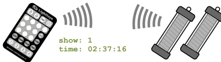
If some FT device doesn't catch the signal, the moment it gets it, it will calculate its precise position in the show (with 2 millisecond accuracy) and start from there!
